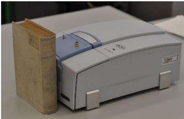
Measurement arrangement using the reflection module of the Bruker Alpha II infrared spectrometer
