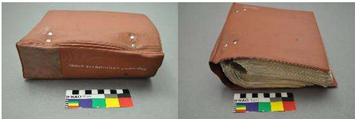
Deformation of boards due to collapse of the spine of the book
