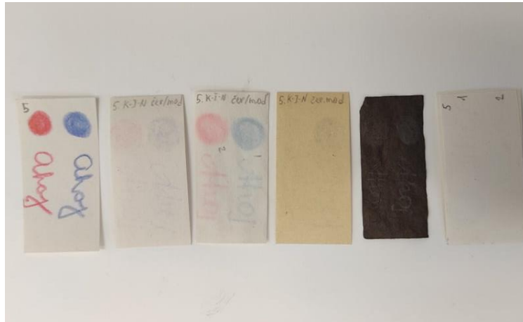
Six samples of Koh-i-Noor Hardtmuth red/blue ink pencil recording medium on Holmen paper. From left: reference sample, mechanical damage, distilled water damage, UV light damage, thermally damaged sample and overglued sample.
