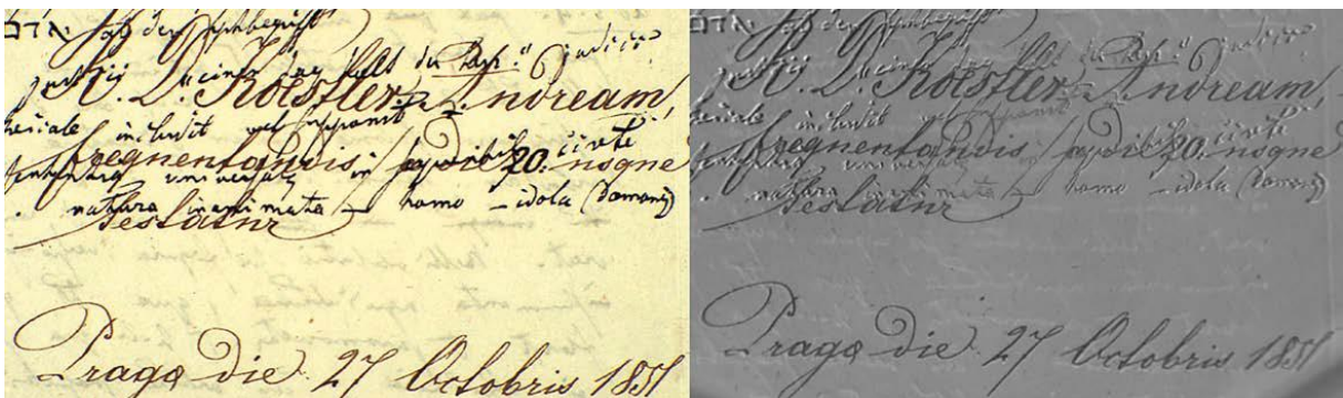
Handwritten document. Observations in incident visible light (left) and in spot lighting 585-720 nm with RG 780 nm short wave filter (right). The text can be read well in the chosen lighting.
