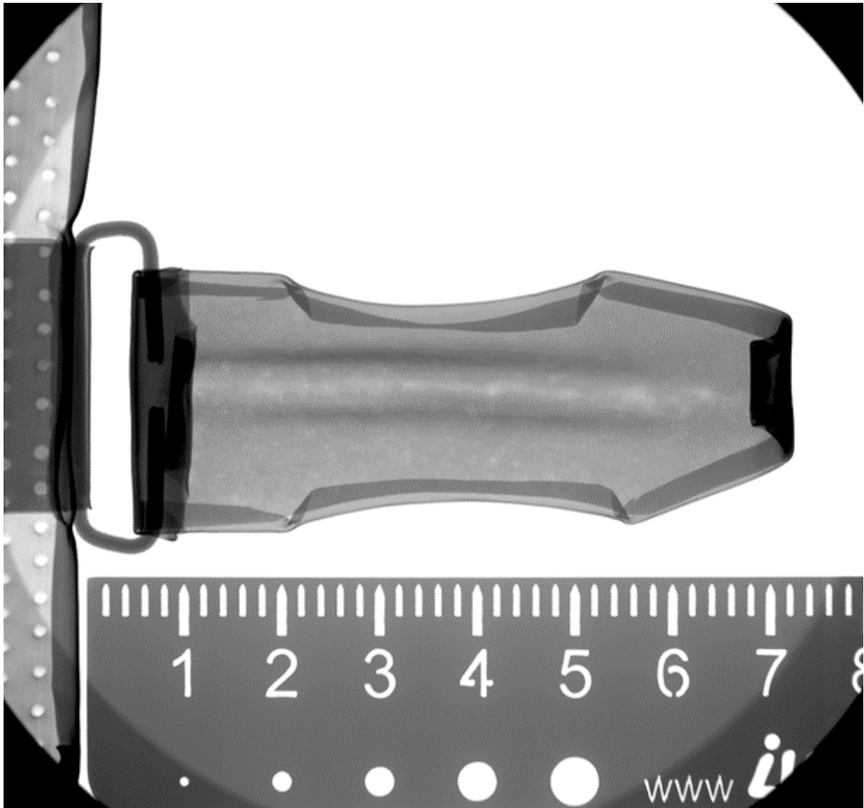
A detail of the ironwork of the book Nebeklič . The buckle closure has a core made from material 3 mm thick; its face is covered with a thin metal sheet that also covers the book cover. A thin metal sheet folded over the core is clearly visible in the image. We can also see that the metal element connecting the clasp to the book cover does not show signs of significant corrosion damage.
