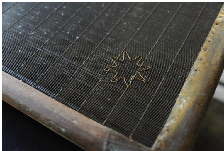
Wire sewn to the sieve of a papermaking frame.
