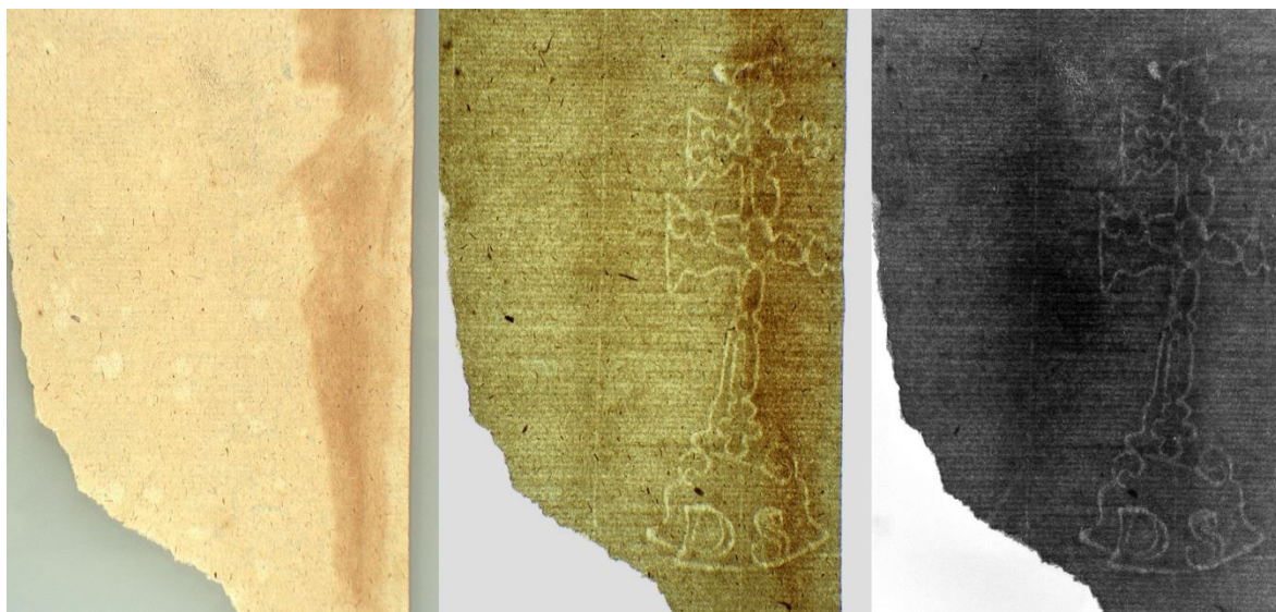
Fragment of a sheet with a watermark. Observations in incident VIS (left), in lower diffused light (centre) and in incident VIS with RG925 short wave pass filter (right) – negative display.
